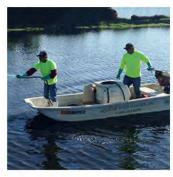
Skiffs are small boats that are equipped with trolling motors and specialized equipment. They are ideal for larger ponds where the weeds are too far away from the shoreline to be reached by a backpack or an ATV.
