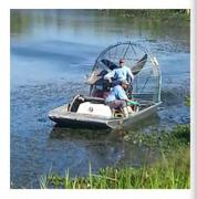
An **airboat** can navigate easily through shallow swamps and marshes. They can travel over and through patches of invasive plants where a regular boat propeller would get entangled.
